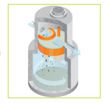
In 2001, Peterborough chose the Stormceptor oil and sediment separator (OGS) because it had been tested and verified to remove and retain more pollutants from stormwater than any other OGS separator, treating the broadest range of sediment particle sizes, as well as
